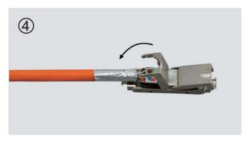
4. Place wiring cap assembly into the cable joiner. Close the cover and repeat for the second cable.
