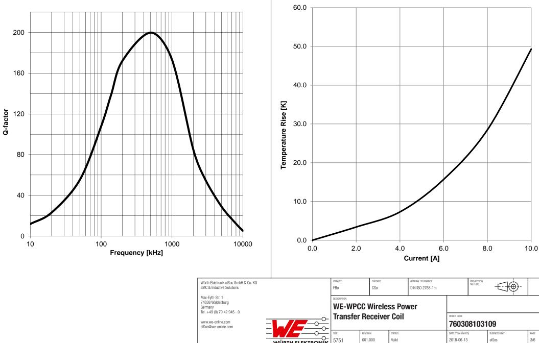
**Typical Temperature Rise vs. Current Characteristics:**
