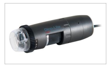
The wide range of magnification (10-140x), the large field of view and working distance of up to 23 cm makes the AM4115ZTL the ideal solution for all situations where a longer distance between the microscope and the object is required or when it is needed to work under the microscope (repair, rework and assembly tasks etc.) The built-in adjustable polarizer reduces glare and reflection on shiny objects.
