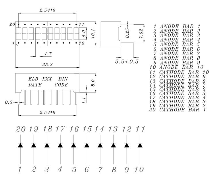
Notes: 1.All dimensions are in millimeters , tolerance is 0.25mm unless otherwise noted.2.Above specification may be changed without notice.Supplier will reserve authority on material change for above specification.
