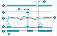
When the HSV has been configured in "memory" mode, if underspeed is detected, the output relay stays in the rest state ("alarm") irrespective of any subsequent change in the speed of the process.
