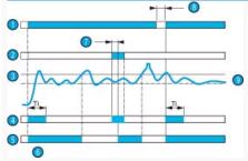
When the HSV has been configured in "memory" mode, if overspeed is detected, the output relay stays in the rest state ("alarm") irrespective of any subsequent change in the speed of the process. It will not be able to revert to ("normal") operating state until contact S2 closes (50 ms minimum). If, when S2 reopens, the speed is too high, the relay reverts to the rest latched state ("alarm").
