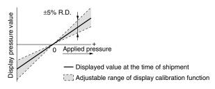
Note) When the precision indicator setting function is used, set pressure value may change  $\pm 1$  digit.
