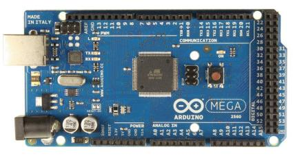
connect it to a computer with a USB cable or power it with a AC-to-DC adapter or battery to get started. The Mega is compatible with most shields designed for the Arduino Duemilanove or Diecimila.
