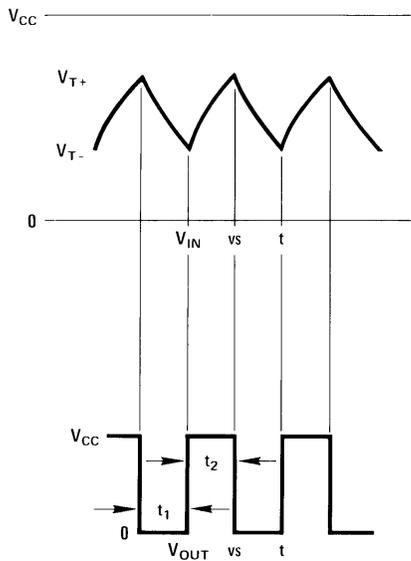
$$f \approx \frac{1}{RC \ln \frac{V_{T+}(V_{CC} - V_{T-})}{V_{T-}(V_{CC} - V_{T+})}}$$
