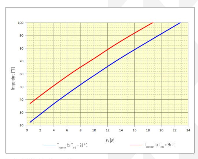
Tested with Mini-ItX Board Core I7 processor 4770.
