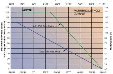
Example: At  $300^{\circ}$ C, the maximum power of a  $0.010^{\circ}$  mica heater is  $70 \text{ W/in}^2 (10.9 \text{ W/cm}^2)$ .
