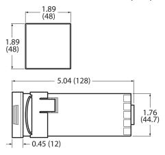
PANEL CUTOUT:  $1.775" \times 1.775" (45 \text{ mm} \times 45 \text{ mm})$ MAXIMUM PANEL THICKNESS: 0.25" (6.35 mm)
