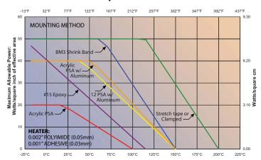
Example: At  $50^{\circ}$ C, the maximum power for a heater mounted with acrylic PSA is  $18 \text{ W/in}^2$  (2.79 W/cm<sup>2</sup>).
