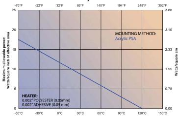
Example: At -20°C, the maximum power for a Thermal-Clear mounted with acrylic PSA is  $14 \text{ W/in}^2 (2.17 \text{ W/cm}^2)$ .
