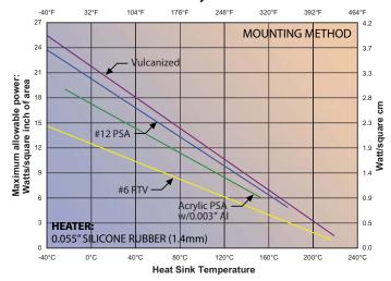
Example: At  $100^{\circ}$ C, the maximum power of a heater mounted with #6 RTV is 7 W/in<sup>2</sup> (1.09 W/cm<sup>2</sup>).
