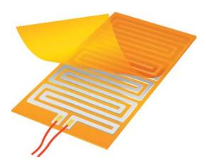
Thermofoil™ heaters are thin, flexible components consisting of an etched-foil resistive heating element laminated between layers of flexible insulation. Since their introduction by Minco over 45 years ago, Thermofoil heaters have demonstrated significant advantages over conventional electric heaters.
