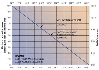
Example: At  $150^{\circ}$ C, the maximum power of a factory-mounted AP heater is  $50 \text{ W/in}^2$  (7.75 W/cm²).
