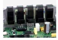
Bergquist Sil-Pad A1500 is a silicone-based, thermally conductive and electrically insulating material. It consists of a cured silicone elastomeric compound coated on both sides of a fiberglass reinforcement layer.
