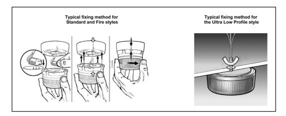
If a higher IP rating is required, a Weatherproof Cable Connector is available, designed to upgrade our Standard and Fire style beacons to IP67 for outdoor/storm applications. Two versions are available, for AC (Part No. 45-710001) and DC (Part No. 45-710002) types.
