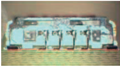
Cross Section Right Angle Male Connector
