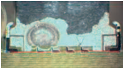
Cross Section Vertical Male Connector
