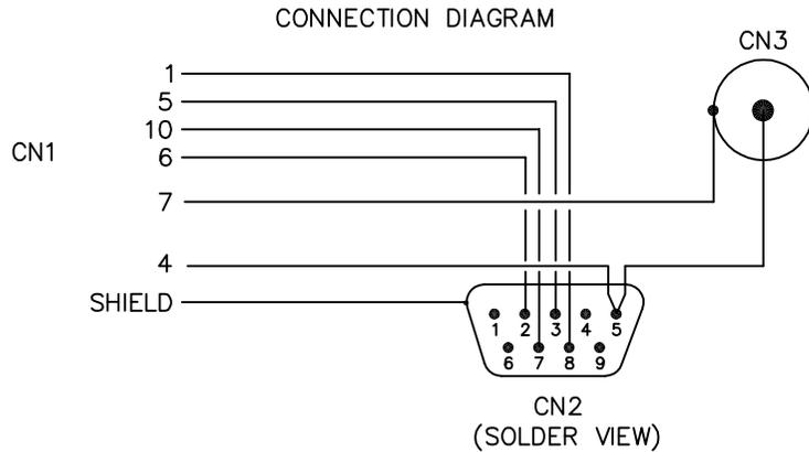
NOTE: connect the housing to the shield of the cable
