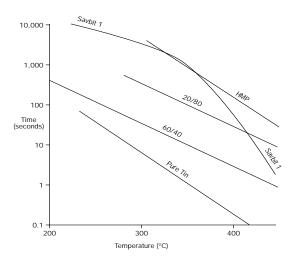
Savbit solder has been used by leading electronics manufacturers throughout the world for over forty years. Savbit was originally used to increase the life of copper soldering iron bits. Soldering speed and efficiency are increased by keeping the iron in good condition. Ironplated bits having a longer life than plain copper tips are now commonly used but they also fail eventually (usually by cracking of the plating) and then erode rapidly unless Savbit solder is used.
