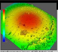
Interferometer image of 3D debris and contamination (courtesy of FiBO)
