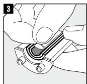
Adapt the seal to the cable/pipe by peeling layers from the halves until you reach the gap seen in pic.4.
