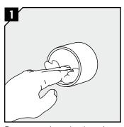
Remove any dirt in the sleeve/hole.
