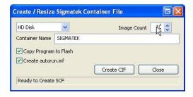
Under "Container Name", a user-defined container name can be assigned. Under "Number of images", the number of "diskettes" for which the Compact Flash is configured can be defined.
