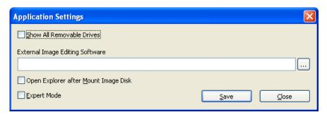
When the control box "Show all removable Drives" is activated, the program detects all removable drives using the manufacturer/product description (system manager). This is then shown in the program window under "removable drives" and the desired Compact Flash can be selected.
