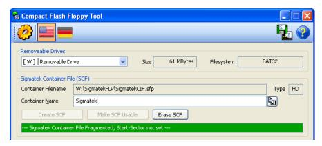
So that a Compact Flash can be used for a Sigmatek container file, a "start sector" must be set. If a start sector cannot be set, the Compact Flash must be defragmented (recommended: HDiskDefrag von http://www.withopf.com/tools/hdiskdefrag).
