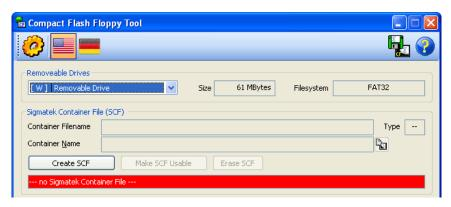
The drive description (i.e.: drive W), capacity (61 Mbytes) and file system (FAT32) of the compact flash card is displayed.
