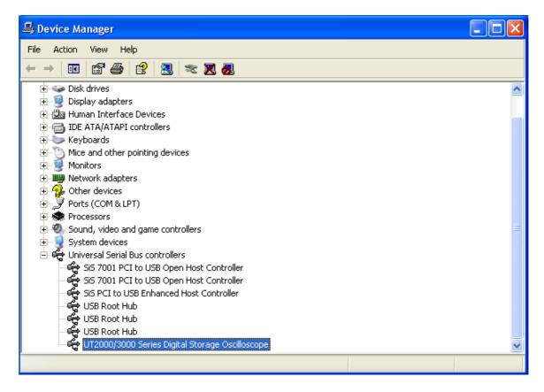
Note: If no [Found New Hardware] wizard pops up on your computer screen when the computer is properly connected to the oscilloscope and the latter is powered on normally, right click [My Computer] and select [Attribute]. In the [System Attribute] dialogue box select the [Hardware] box. Click the [Device Manager] button.
