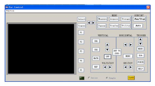
Important: The above screen will not display waveform. Operation of this screen will be indicated in the oscilloscope.
