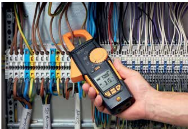
Measuring current in a switching cabinet.
