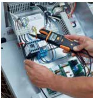
Measuring voltage on a compressor.
