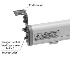
Note) The number of centre brackets required, as listed below, depends on the bar length. Two end brackets are always required regardless of the bar length.
