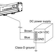
\* DC1 (-) [Blue] is sure to ground it according to class-D. If the terminal is not grounded, the ionizer may malfunction.
