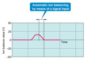
The ion balance is not affected by the height of installation or any disturbance interference since the ionizer is designed to adjust the ion balance near the autobalance sensor.
