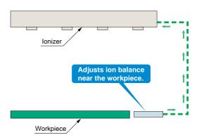
• The autobalance sensor may be connected only when adjusting the ion balance.
