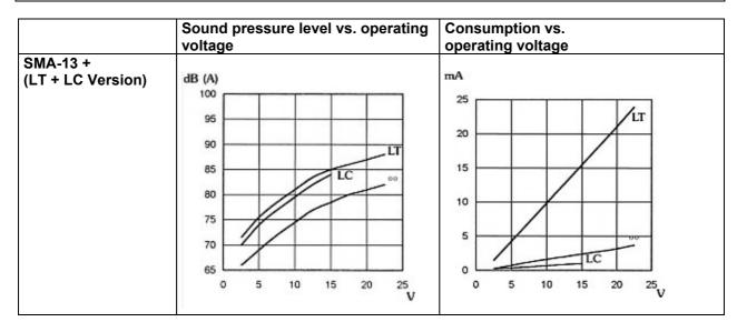
All measurements are made at 30 cm in free air at 21°C.
