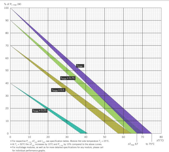
•  $\Delta T$  = Hot side temperature ( $T_p$ ) less Cold side temperature ( $T_c$ ).
