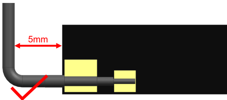
FIGURE 5.2.1 RECOMMENDED CABLE BENDING RANGE
