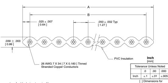
Note: Red marking on one edge of cable designates wire #1.
