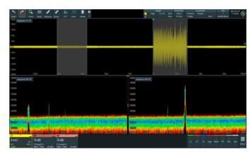
The gated FFT function of the R&S®RTO6 oscilloscope applies FFT analysis only to user-defined regions of the acquired time domain signal.
